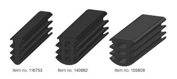
The milled groove of the optical guidance system must be sealed against environmental conditions. A simple and low-cost solution is to use the halogen-free GIFAS system profile made of EPDM. This is inserted in the slot. It is self-locking and available in three different widths. A stable and smooth slot with slot widths of 6 -15 mm is the prerequisite for use.
